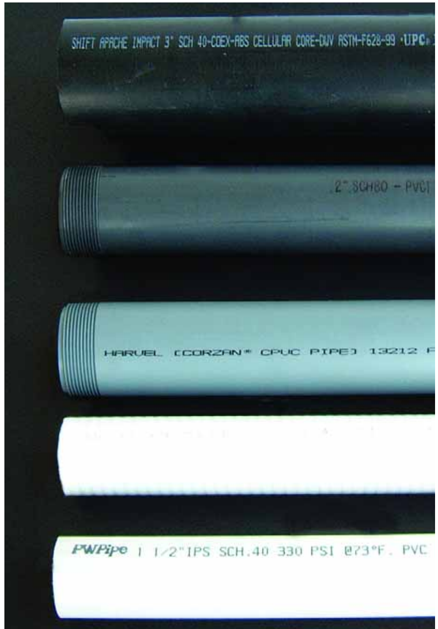
Figure 1: The five most common types of pipe used for swimming pool plumbing are, from top to bottom, ABS, schedule 80 PVC, CPVC, PVC Flex and rigid Schedule 40 PVC.
