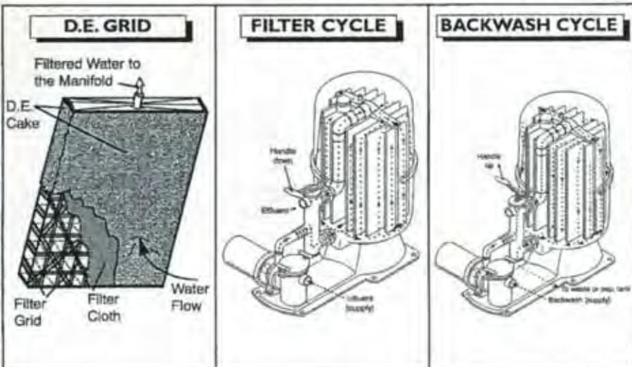
In commercial applications, systems can include auto-backwash valves equipped with special slurry-feed systems that add D.E. to the filter after it's been cleaned.)
