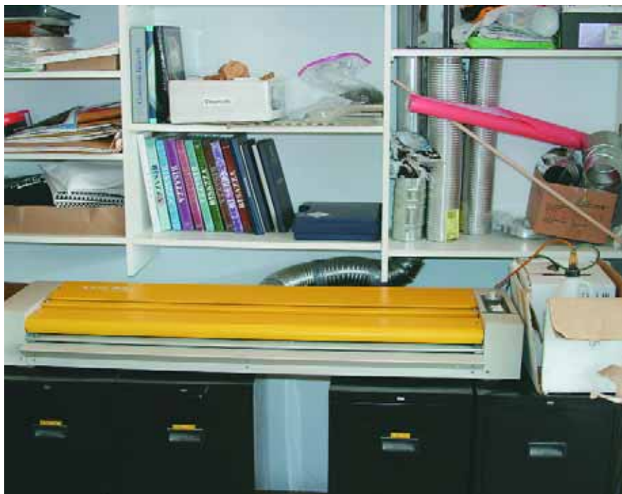
This blueprint machine is a gem. It takes up plenty of space and requires lots of ventilation, but it gives me the ability to generate my finished drawings in whatever form or format is required – blue lines, brown lines, sepias, acetates or vellums.
