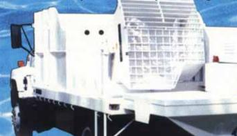
Pumps up to 500 feet of material hose, and up to 400 sacks per day.
